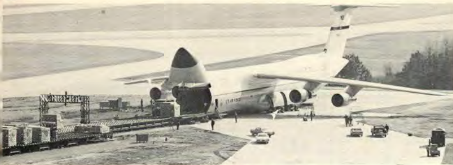
Palletized cargo rolls from the newly developed Air Transportable Dock onto a C-5 at Marietta, Ga., for flight to Pope AFB/Ft. Bragg, NC. The dock can be transported by C-5 Galaxys to forward areas, off-loaded and set up to handle arriving palletized supplies.
